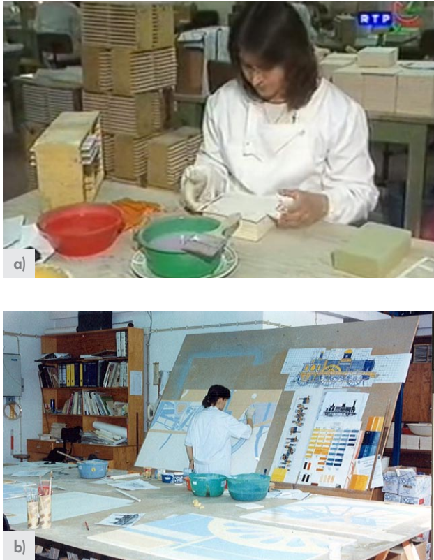
Fig. 02. Azulejo painting at Constância Factory: a) Stencilling (Video frame, available at: https://www.youtube.com/watch?v=zklisKTYTjQ (2017.02.01) and b) Manual panel painting (archive of the interviewed Paulo Matos).
